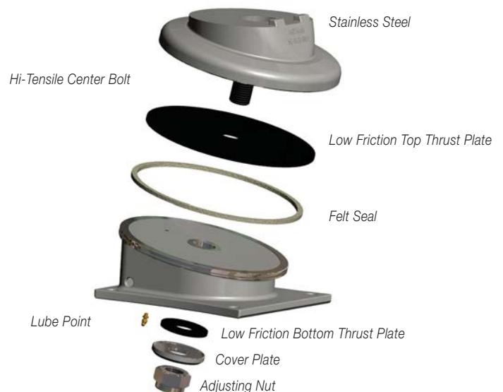
TuffTrak Centre Pivots - Complete Bearing Assembly
